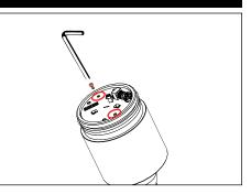
Use a 5/64" allen wrench to remove two (2) #2-56 3. socket head cap screws on LED board, grasp LED board and gently pull up to expose quick disconnect
