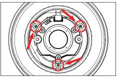
Use a .050" allen wrench to loosen three (3) set 3. screws holding LED module. Gently lift from fixture.
