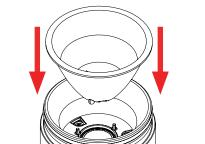
5. Replace optic by lining notches with optic holder, then pressing down gently until secured into place.
