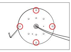
3. Circled locations are mounting holes for mounting heavy duty mounting plate to substrate. Use mounting hardware suitable for substrate material. **Seal building envelope as per NEC.**
