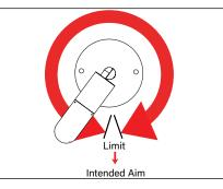
3. If the over-rotation protection pin is in the desired aiming position, do not force the fixture past the limit. Using a 3/16" allen wrench, slightly loosen both set screws in the knuckle, enough to move the fixture freely on both axes.
