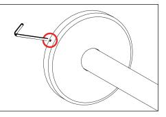
Ensure fixture leads are inside junction box. Mount fixture canopy to junction box over mounting plate using three (3) #8-32 set screws with a 9/64" allen wrench.
