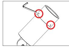
Use a 5/64" allen wrench to slightly loosen 2. Remove optic by pulling gently and lift up. 1. three (3) #8-32 stainless steel set screws to remove cap.
