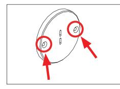
Mount support canopy above fixture location using appropriate mounting hardware for surface. Seal building envelope as per NEC. Do not overtighten.
