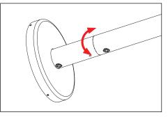
Adjust stem so that cable notch in stem lines up with support canopy location and cable. Loosen 3/8" set screw in stem to adjust.
