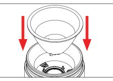
5. Replace optic by lining tabs with optic holder, then pressing down gently until secured into place.
