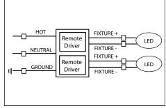
Pull fixture leads through heavy duty mounting plate. Make watertight connections from remote driver to fixture leads using waterproof wire connectors. See wiring diagram. WIRING DIAGRAM - SINGLE FIXTURE
