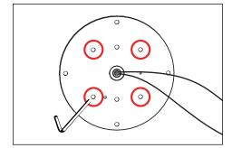
Install mounting plate (included) with #10-24 screws using a 1/8" allen wrench onto back box. Circled locations are available mounting holes for back box installation.
