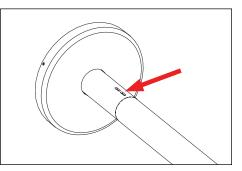
7. Tighten set screw when cable notch in stem is in line with support cable and support canopy.
