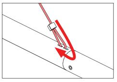
Thread aircraft support cable through cable notch in stem. Loop and fasten with compression fitting. Use proper crimping tool to close compression fitting.
