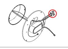
Ground primary branch circuit to wall plate per NEC. 2. Make connections from transformer to primary branch circuit using proper wire connectors. (not included). See wiring diagram.
