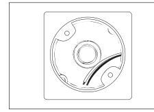
Install mud ring to junction box using appropriate hardware (mud ring, junction box and hardware not included). Align canopy mounting holes to final mounting position.
