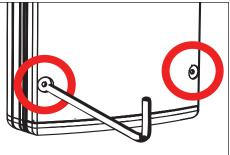
Loosen four (4) #6-32 captive screws using a 5/64" allen wrench and disconnect quick disconnect to remove faceplate of UPM housing.
