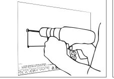
2. Drill holes into surface for ¼" fasteners on locations 3. illustrated on template.
