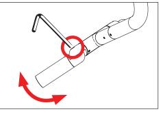
Use a 5/32" allen wrench to loosen #10-32 stainless steel black oxide socket head cap screw at the knuckle. Aim fixture to desired vertical location. Tighten to secure aiming position.
