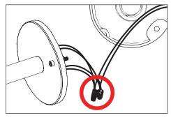
2. Make watertight connections from remote transformer to fixture leads using waterproof wire connectors (not included). See wiring diagram.
