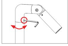
To adjust stem horizontally, loosen two (2) #8-32 screws at base of stem cap using a 5/64" allen 4. wrench. Adjust as needed, then secure.
