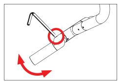
Use a 5/32" allen wrench to loosen #10-32 stainless steel black oxide socket head cap screw at the knuckle. Aim fixture to desired vertical location. Tighten to secure aiming position.
