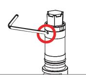
Use a .050" allen wrench to loosen two (2) #4-40 stainless steel set screws below LED board on the heat sink. Gently pull up on LED board and Driver assembly to expose quick disconnect.
