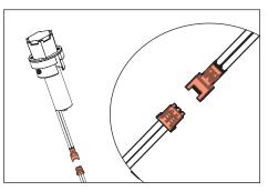
3. Disengage LED board and driver assembly. Replace with new board and driver assembly.
