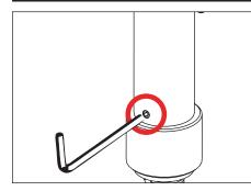
1. Use a 5/64" allen wrench to loosen #8-32 stainless steel set screw and remove cap.
