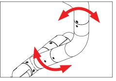
Use a 5/64" allen wrench to loosen #8-32 screws at bend(s). Aim fixture to desired position. Tighten to secure aiming position.
