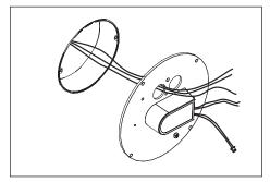
1. Remove one or two wire entrance knockouts on wall plate. Pull primary branch circuit through knockout(s). Attach wall plate to junction box using appropriate hardware (not included).
