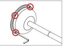
Mount canopy to wall plate using four (4) #8-32 stainless steel button head screws with a 5/64" allen 4. wrench. Seal building envelope as per NEC. Do not overtighten.
