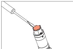
5. Use small flat head screw driver to remove lens from optic holder on the LED. Snap new optic in place. Replace cap on fixture and tighten set screw.
