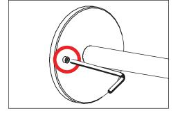
Mount fixture canopy directly to 3" junction box or 4" junction box with mud ring using two (2) #10-24 hex screws using a 1/8" allen wrench. Seal building envelope as per NEC. Do not overtighten.
