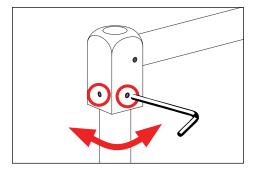
To adjust stem horizontally, loosen two (2) #8-32 screws at base of stem cap using a 5/64" allen wrench. Adjust as needed, then secure.
