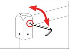
To adjust stem, loosen #8-32 screw with a 5/64" allen wrench at stem cap. Adjust as needed, then secure.
