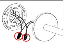
Make watertight connections from remote transformer to fixture leads using waterproof wire connectors (not included). See wiring diagram.
