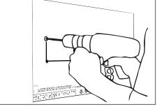
Prepare for final mounting position according to 2. Drill holes into surface for ¼" fasteners. designed lighting plan.
