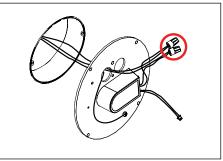
Ground primary branch circuit to wall plate per NEC. Make watertight connections from transformer to primary branch circuit using waterproof wire connectors. See wiring diagram.
