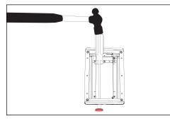
4. Remove Patented Knockout(s) as necessary from the inside of the UPM housing. Leave remaining unused knockouts in place to maintain seal.
