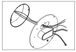
Remove wire entrance knockouts as needed on wall plate. Pull primary branch circuit through knockout(s). Attach wall plate to junction box using appropriate hardware.
