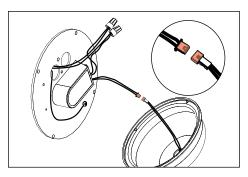
3. Connect fixture to transformer with provided quick disconnect.
