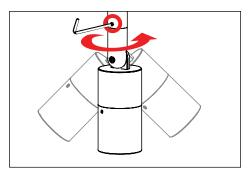
Optional 360SL: Use a 5/64" allen wrench to loosen stainless steel set screw on the 360SL rotational mounting system and rotate to desired horizontal location. Tighten to secure aiming position.
