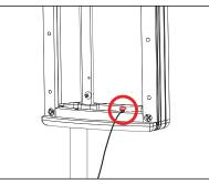
Attach tether wire under screw head at the base of the UPM housing and tighten. Slowly lower the faceplate until tether is taut.
