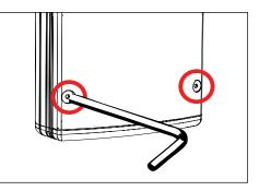
Loosen four (4) #6-32 captive screws using a 5/64" allen wrench and disconnect quick disconnect to remove faceplate of UPM housing.
