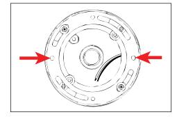
Install universal mounting ring (supplied with fixture) with #10-24 screws using a 1/8" allen wrench onto back box. Align fixture mounting holes to final mounting position.
