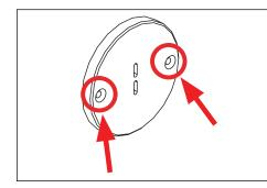
Mount support canopy above fixture location using appropriate mounting hardware for surface. Seal building envelope as per NEC. Do not overtighten.
