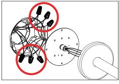
Pull fixture leads through heavy duty mounting plate. Make watertight connections from remote driver to fixture leads using waterproof wire connectors (not included). See wiring diagram.
