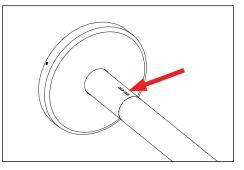
8. Tighten set screw when cable notch in stem is in line with support cable and support canopy.
