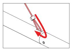
Thread aircraft support cable through support canopy cable notch. Loop and fasten with compression fitting. Use proper crimping tool to close compression fitting.
