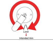
If the over-rotation protection pin is in the desired aiming position, do not force the fixture past the limit. Using a 3/16'' allen wrench, slightly loosen 3. both set screws in the knuckle, enough to move the fixture freely on both axes.
