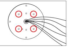
Install mounting plate (included with fixture) with #10-24 screws using a 1/8" allen wrench onto back box. Circled locations are available mounting holes for back box installation.
