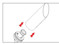
Loosen #8-32 stainless steel set screw with a 5/64" 1. allen wrench on cap. Retain screw in cap.
