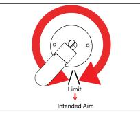
If the over-rotation protection pin is in the desired aiming position, do not force the fixture past the limit. Using a 5/64" and 5/32" allen wrench, slightly loosen both set screws in the knuckle and knuckle screw enough to move the fixture freely on both axes.
