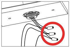
3. Make watertight connections from primary branch circuit wiring to fixture leads using waterproof wire connectors. Connect incoming ground to green ground wire from fixture. **See wiring diagram.**
