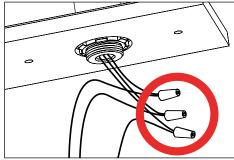
Make watertight connections from primary branch circuit wiring to to lamp leads using waterproof wire connectors (not included). Ground incoming ground wire to ground wire from fixture. See wiring diagram.
