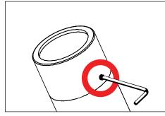
1. Use a 5/64" allen wrench to loosen #8-32 stainless set screw and remove cap.
