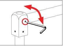
5. To adjust stem, loosen #8-32 screw with a 5/64" allen wrench at stem cap. Adjust as needed, then secure.
