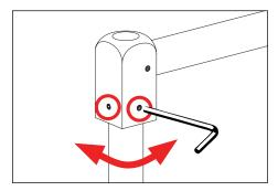
4. To adjust stem horizontally, loosen two (2) #8-32 screws at base of stem cap using a 5/64'' allen wrench. Adjust as needed, then secure.
