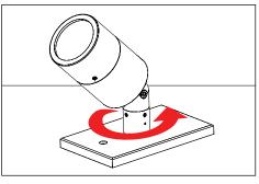
2. Rotate fixture at base and aim fixture to desired horizontal location.
