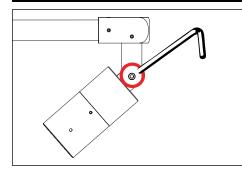
Use a 5/32" allen wrench to slightly loosen #10-1. 32 stainless steel set screw on the stem for 180° aiming purpose.
