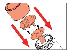
Reverse install LED board and driver by carefully wrapping 18 gauge wires around driver and inserting into fixture body. Secure LED board in place with stainless steel screws.
