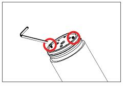
Use a 5/64" allen wrench to remove two (2) #2-56 socket head cap screws on LED board, grasp LED board and gently pull up to expose quick disconnect.
