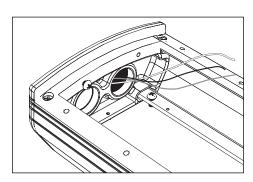
7. Pull branch circuit wiring necessary for installation.
