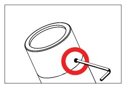
With flat head screw driver rotate dial to desired lumen output. Replace cap.
