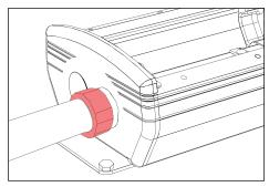
Connect 3/4" conduit connector through female threaded conduit entry.
