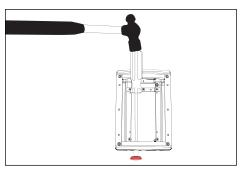
Remove Patented Knockout(s) as necessary from the inside of the UPM housing. Leave remaining unused knockouts in place to maintain seal.
