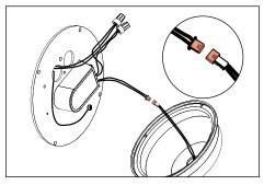
Connect fixture to transformer with provided quick disconnect.
