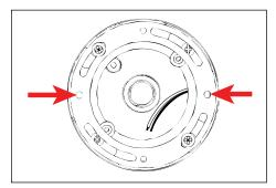
Install universal mounting ring (included with fixture) with #10-24 screws using a 1/8" allen wrench onto back box. Align fixture mounting holes to final mounting position.
