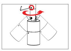
Optional 360SL: Use a 5/64" allen wrench to loosen stainless steel set screw on the 360SL rotational mounting system and rotate to desired horizontal location. Tighten to secure aiming
