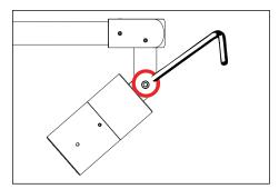
Use a 5/32" allen wrench to slightly loosen #10-32 stainless steel set screw on the stem for 180° aiming purpose.
