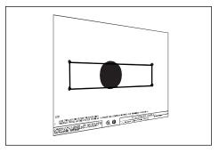
Prepare for final mounting position according to 2. Drill holes into surface for ¼" fasteners. designed lighting plan.
