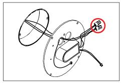
Ground primary branch circuit to wall plate per NEC. Make watertight connections from transformer to primary branch circuit using waterproof wire connectors. See wiring diagram.
