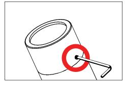
Place cap on fixture and tighten set screw. Tighten screw to 1/2 in-lbs. Top of screw should sit flush with fixture cap.
