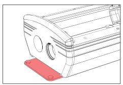
Attach the UPM housing at mounting brackets with 1/4" fasteners. Use suitable mounting hardware for
