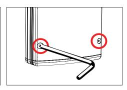
Loosen four (4) #6-32 captive screws using a 5/64" allen wrench and disconnect quick disconnect to remove faceplate of UPM housing.
