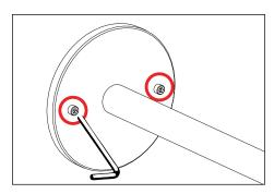
Mount canopy to junction box with universal mounting ring using two (2) #10-24 stainless steel black oxide screws with a 1/8" allen wrench. Seal building envelope as per NEC. Do not overtighten.
