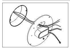
Remove wire entrance knockouts as needed on wall plate. Pull primary branch circuit through knockout(s). Attach wall plate to junction box using appropriate hardware.
