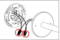
Make watertight connections from remote transformer to fixture leads using waterproof wire connectors. See wiring diagram.
