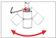
4. Use a 5/32" allen wrench to loosen #10-32 stainless steel black oxide socket head cap screw at the knuckle. Aim fixture to desired vertical location. Tighten to secure aiming position.
