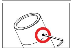
Use a 5/64" allen wrench to loosen #8-32 stainless set screw and remove cap.
