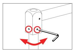
To adjust stem horizontally, loosen two (2) #8-32 screws at base of stem cap using a 5/64" allen wrench. Adjust as needed, then secure.
