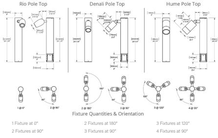
Shown with four Denali Integral Fixtures at  $90^\circ$
