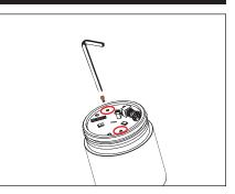
Use a 5/64" allen wrench to remove two (2) #2-56 3. socket head cap screws on LED board, grasp LED board and gently pull up to expose quick disconnect.
