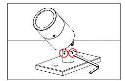
Use a 5/64" allen wrench to slightly loosen two (2) #8-32 stainless steel set screws on the stem for 360° aiming purpose.
