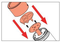
Reverse install LED board and driver by carefully wrapping 18 gauge wires around driver and inserting into fixture body. Secure LED board in place with stainless steel screws.
