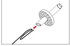
Loop 12" of low voltage wire inside power pipe. Do not remove temporary cover.
