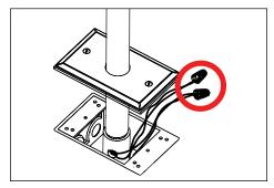
Make watertight connections from remote 12V transformer to fixture leads using waterproof wire connectors. See wiring diagram.
