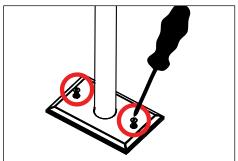
Attach box cover to junction box by tightening two (2) #6-32 stainless steel slotted screws to secure.
