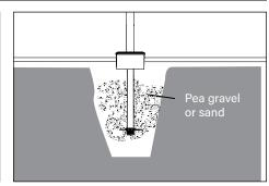
Back fill with pea gravel or sand prior to pour. Junction box can be installed above or below grade level
