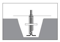
Pull low voltage wiring from remote 12V transformer to power pipe. Allow for additional cable to make connections to fixture lead and future service. Place power pipe in hole.
