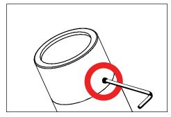
With flat head screw driver rotate dial to desired lumen output. Replace cap.
