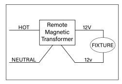
Make watertight connections from remote 12V transformer to lamp leads (18 gauge wire) using waterproof wire connectors. See wiring diagram.
