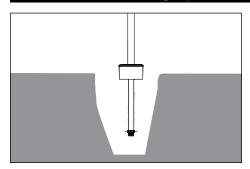
Excavate trench according to designed lighting plan. Dig hole a minimum of 18" deep and 10" wide to accommodate anchor base at desired fixture locations.
