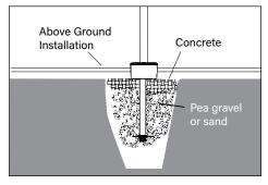
5. For above ground installation. Pour concrete below junction box.
