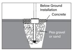
For below ground installation. Pour concrete to 7. grade and flush with junction box.
