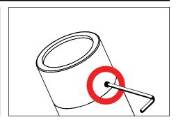
3. Place cap on fixture and tighten set screw. Tighten screw to 1/2 in-lbs. Top of screw should sit flush with fixture cap.
