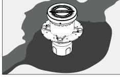
Place housing in hole. Align junction box in the path of the conduit trench.
