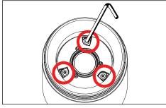
Use a .050" allen wrench to loosen three (3) set screws holding optic holder and LED module.
