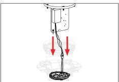
Connect the faceplate with the driver assembly to installed HydroLock with factory wired quick connectors. Lower faceplate assembly into HP2 busing
