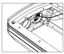
7. Pull branch circuit wiring and dimming control wiring necessary for installation (By Others.)
