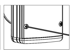
Make sure UPM housing gasket is free of any dirt or debris. Attach the faceplate by tightening the (6) #10-24 captive screws evenly using a 1/8" Allen wrench.
