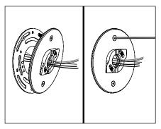
4. Feed branch circuit wiring and dimming control wiring through mounting plate with CamLock™ assembly. Attach mounting plate with supplied (2) #10-24 stainless steel hex drive fasteners to universal ring using 1/8" Allen wrench.
