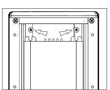
Remove two (2) #8-32 screws in UPM housing using Phillips screwdriver.
