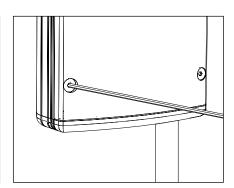
13. Make sure UPM housing gasket is free of any dirt or debris. Attach the faceplate by tightening the (6) #10-24 captive screws evenly using a 1/8" Allen wrench.
