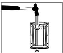
2. Remove Patented Knockout(s) as necessary from the inside of the UPM housing. Leave remaining unused knockouts in place to maintain seal.
