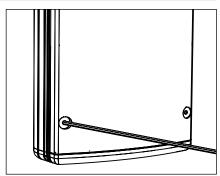
Loosen (6) #10-24 captive screws using a 1/8" Allen wrench to remove faceplate of UPM housing.
