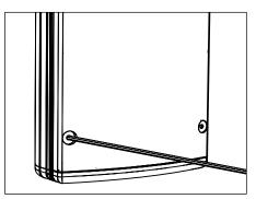
Loosen (6) #10-24 captive screws using a 1/8" Allen 1. wrench to remove faceplate of UPM housing.
