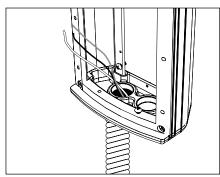
Pull branch circuit wiring and dimming control wiring necessary for installation (By Others).
