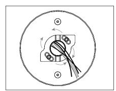
If UPM housing is not level, remove UPM housing; loosen but **DO NOT REMOVE** (2) #8-32 screws with 9/64" Allen wrench on CamLock™ assembly. Adjust CamLock™ assembly up to 30° as needed to level. Tighten the screws and reattach UPM housing.
