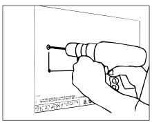
Drill holes into surface for ¼" fasteners (By Others) on locations illustrated on template.
