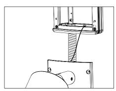
Attach tether wire under screw head at the base of the UPM housing and tighten. Slowly lower the faceplate until tether is taut.
