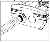
Connect 3/4" conduit connector through 6. female threaded conduit entry.
