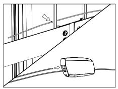
Thread safety cable through hole on the back of the UPM housing. Feed safety cable through opposing ends of the connector. Pull on wires to assure the connection is secure. Leave enough slack in safety cable for tree growth. Adjustments can be made by pressing release spring with a pin or 3/64" Allen
