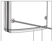
Make sure UPM housing gasket is free of any dirt or debris. Attach the faceplate by tightening the (6) #10-24 captive screws evenly using a 1/8" Allen wrench.
