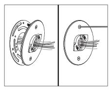
Feed branch circuit wiring and dimming control wiring through mounting plate with CamLock™ assembly. Attach mounting plate with supplied (2) #10-24 stainless steel hex drive fasteners to universal ring using 1/8" Allen wrench.
