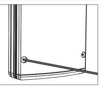
Loosen (6) #10-24 captive screws using a 1/8" Allen wrench and disconnect quick disconnect to remove faceplate of UPM housing.
