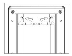
10. Remove two (2) #8-32 screws in UPM housing using Phillips screwdriver.
