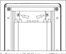
9. Remove two (2) #8-32 screws in UPM housing using Phillips screwdriver.
