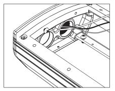
7. Pull branch circuit wiring and incoming dimming control wiring necessary for installation (By Others.)
