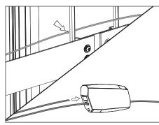
Thread safety cable through hole on the back of the 4. UPM housing. Feed safety cable through opposing ends of the connector. Pull on wires to assure the connection is secure. Leave enough slack in safety cable for tree growth. Adjustments can be made by pressing release spring with a pin or 3/64" Allen tool.
