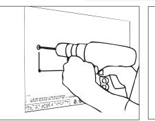
2. Drill holes into surface for ¼" fasteners (By Others) on locations illustrated on template.
