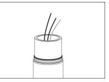
Pole in mounting plate has 2-3/8" O.D. and is 5-1/4" 3. Pull branch circuit wiring needed, through pole tenon.
