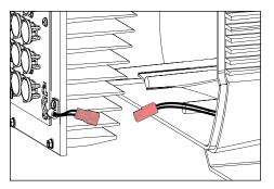
3. Use quick disconnect to disconnect heatsink and LED board from driver.
