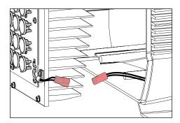
7. Reconnect quick disconnect from driver secondary side to LED board assembly.
