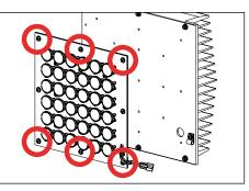
4. If replacing LED board: Remove LED board and thermal pad from heatsink by loosening sixteen (16) Phillips screws using Phillips screwdriver. Line up new thermal pad and LED board on heatsink. Replace board and thermal pad on heatsink with thermal pad closest to heatsink, then reverse install.
