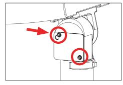
7. Attach wiring compartment access panel to knuckle wiring compartment by tightening two (2) screws using 5/16" socket wrench.
