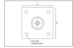
Prepare for installation for mounting plate. 2. Mounting plate has four (4) 9/16" dia. mounting holes (Mounting Hardware by Others) in a 6" bolt 1. circle.
