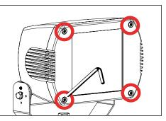
Replace faceplate by tightening four (4) tamperresistant hex screws using a Torx T27 tamper resistant hex bit.
