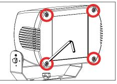
1. Remove faceplate by loosening four (4) tamperresistant hex screws using a Torx T27 tamper resistant hex bit.
