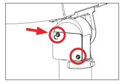
4. Remove wiring compartment access panel to knuckle wiring compartment by loosening two (2) screws using 5/16" socket wrench.
