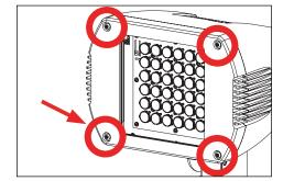
To relamp: remove faceplate and louver by loosening four (4) tamper resistant screws using a TORX T27 socket (1/4" bit). Relamp as needed, then reverse install.
