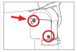
Remove wiring compartment access panel to knuckle wiring compartment by loosening two (2) screws using a 5/16" socket wrench.
