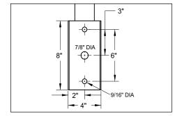
1. Prepare location for wall pole mounting arm. Wall pole mounting arm bracket is 4" wide, clearance holes 2" from side. Mounting arm bracket is 8" tall, with two 9/16" clearance holes 6" apart on center. Wire way in center of mounting bracket is 7/8" diameter.
