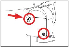
6. Attach wiring compartment access panel to knuckle wiring compartment by tightening two (2) screws using 5/16" socket wrench.
