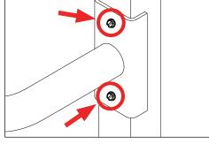
2. Pull branch circuit wiring needed, then install proper mounting hardware for wall pole mounting arm (hardware not included).
