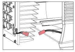
Reconnect quick disconnect from driver secondary side to LED board assembly.
