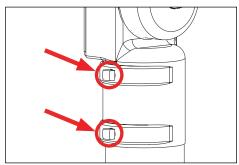
Fit fixture over pole tenon and ensure it is completely seated. Secure fixture to tenon by tightening two (2) 3/8"x16 stainless steel square screws using an adjustable crescent wrench.
