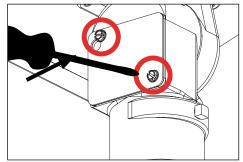
Attach wiring compartment access panel to knuckle wiring compartment by tightening two (2) screws using a 5/16" socket wrench or flat head
