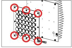
. If replacing LED board: Remove LED board and thermal pad from heatsink by loosening sixteen (16) Phillips screws using Phillips screwdriver. Line up new thermal pad and LED board on heatsink. Replace board and thermal pad on heatsink with thermal pad closest to heatsink, then reverse install.
