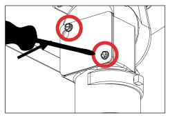
Remove wiring compartment access panel to knuckle wiring compartment by loosening two (2) screws using 5/16" socket wrench or flat head screw driver.
