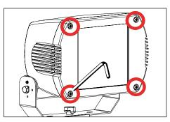
Remove faceplate by loosening four (4) tamperresistant hex screws using a Torx T27 tamper resistant hex bit.
