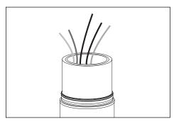
Install pole with standard 2" tenon mount (2-3/8" outer diameter) according to manufacturer's instructions. (Pole By Others). Pull incoming primary branch circuit wiring and external dimming controls.
