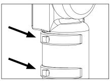
Fit fixture over pole tenon and ensure it is completely seated. Secure fixture to tenon by tightening two (2) 3/8"x16 stainless steel З. square screws using an adjustable crescent wrench.
