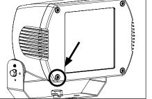
Remove faceplate by loosening four (4) 1. tamper-resistant hex screws using a Torx T27 tamper resistant hex bit.
