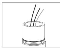
Install pole with standard 2" tenon mount (2-3/8" outer diameter) according to manufacturer's instructions (pole not 1. incuded). Pull incoming primary branch circuit wiring.
