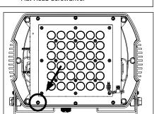
2. Prepare to remove LED board, thermal pad and heatsink by loosening six (6) #8-32 slotted screws using a 1/4 nut driver/socket wrench or a flat head screwdriver.
