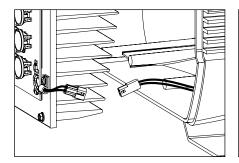
3. Use quick disconnect to disconnect heatsink and LED board from driver.
