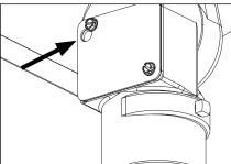
Attach wiring compartment access panel to knuckle wiring compartment by tightening two (2) screws using a 5/16" socket wrench. 5.
