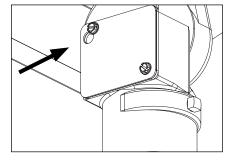
Remove wiring compartment access panel to knuckle wiring compartment by loosening two (2) screws using a 5/16" socket wrench. 2.
