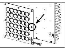
4. If replacing LED board: Remove LED board and thermal pad from heatsink by loosening sixteen (16) Phillips screws using Phillips screwdriver. Line up new thermal pad and LED board on heatsink. Replace board and thermal pad on heatsink with thermal pad closest to heatsink, then reverse install,
