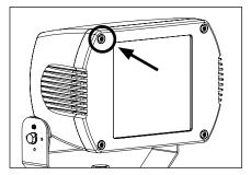
9. Replace faceplate by tightening four (4) tamper-resistant hex screws using a Torx T27 tamper resistant hex bit.
