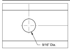
1. Prepare for installation for yoke location. Clearance hole is 9/16" diameter.
