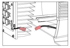
Use quick disconnect to disconnect heatsink and LED board from driver.
