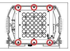
Prepare to remove LED board, thermal pad and heatsink by loosening six (6) #8-32 slotted screws using a 1/4 nut driver/socket wrench or a flat head screwitting.
