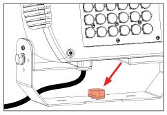
Line up fixture yoke to mounting location and secure with 3/4-10 hex bolt with adjustable crescent wrench.
