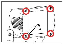
Replace faceplate by tightening four (4) tamperresistant hex screws using a Torx T27 tamper resistant hex bit.
