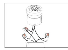
4. Disconnect driver assembly from fixture body.
