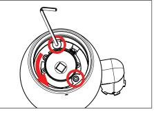
. Rotate the two (2) 8-32 flat head cap screws using a 3/32" allen wrench clockwise until they bottom out into the heatsink, then rotate the heatsink so the screws line up with the grooves. Remove the two (2) 8-32 flat head cap screws from the heatsink completely.
