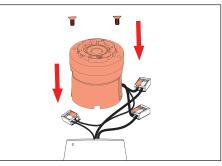
Connect new driver assembly to fixture leads. Place connections inside body cavity, reinsert new heatsink assy back into body. Reinstall two (2) 8-32 flat head cap screws completely onto the heatsink until screws catch under the groove on the body. Rotate the two (2) 8-32 flat head cap screws counterclockwise until they are snug against the top of the groove.
