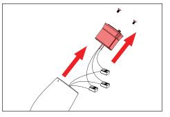
3. Disengage LED board and driver assembly.
