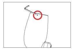
1. Use a 1/16" allen wrench to loosen #6-32 stainless 2. set screw and remove cap.
