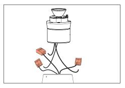
4. Disconnect driver assembly from fixture body.
