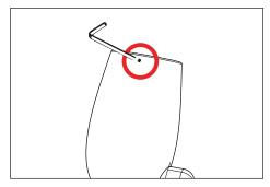
Place cap on fixture and tighten set screw. Tighten screw to 1/2 in-lbs. Top of screw should sit flush with fixture body.
