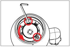
Rotate the two (2) 8-32 flat head cap screws using a 3/32" allen wrench clockwise until they bottom out into the heatsink. Then rotate the heatsink so the screws line up with the grooves. Remove the two (2) 8-32 flat head cap screws from the heatsink completely.
