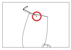
1. Use a 1/16" allen wrench to loosen #6-32 stainless set screw and remove cap.
