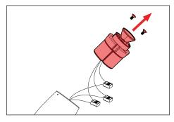
3. Disengage laser board and driver assembly.
