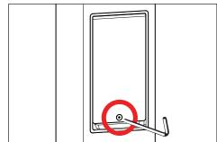
Receptacle cover has captive #6-32 screw. Secure receptacle by tightening captive #6-32 set screw using a 7/64" allen wrench.
