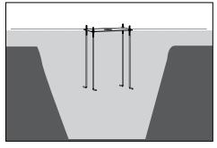
With the conduits in place and the anchor plate properly positioned, secured and leveled, concrete may be poured.
