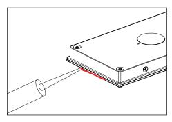
4. Seal as per NEC with waterproof silicone sealant 5. (not included).
