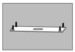
The fixture may be installed by removing the four (4) 1/4-20 nuts and re-using them to secure the fixture mounting base assembly. Trim conduit as needed.
