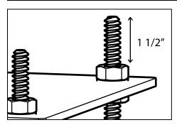
Adjusted anchor bolts to project at least 1-1/2" using the four (4) 1/4-20 nuts to the top of the plate. The four (4) nuts can be left in place while concrete is poured.
