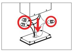
Pull primary branch circuit wiring and any additional dimming controls or other wiring necessary for installation. Attach ground from branch circuit to ground lead on the anchor base. Place connectors inside of the housing (Please refer to page 4 for wiring diagram).
