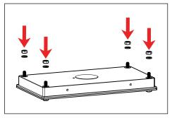
Line up then place base over installed 1/4-20 nuts.
