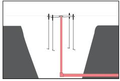
Run conduit inside of the anchor plate center hole prior to pouring concrete.
