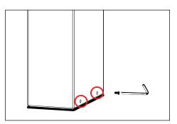
Attach receptacle to installed anchor base with four
