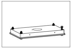
Secure to anchor bolts with the 1/4-20 nuts and lockwashers provided with the YKB Anchor kit using a socket.
