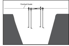
Install anchor plate and bolt assembly flush with 3. the finished grade.
