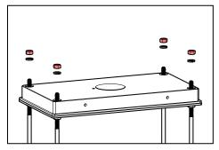
Remove 1/4-20 nuts from installed YKB anchor kit with a socket. Keep the hardware to reuse in the next sten.
