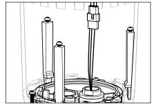
5. Connect optilock assembly to Patented HydroLock Barrier plate with quick disconnect.
