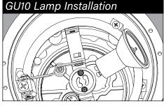
2d. Firmly insert proper GU10 lamp pins into socket, then gently twist to make connection.
