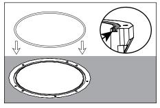
Remove any dirt or debris in o-ring groove near 3. top of housing. Place o-ring inside of groove.
