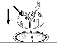
Place OptiLock in HP2 housing and align keyhole notch under one of three (3) #8 screw heads. Rotate horizontally to desired aiming position, then tighten two (2) #8 Phillips screws using Phillips screwdriver. Install proper MR16 halogen, PAR36/AR111, PAR20/30, or GU10 lamp according to instructions on Lamp Installation Or Re-Lamping page.
