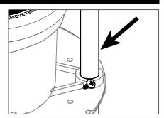
Insert four (4) pieces of ½" EMT conduit through the Stability Flange. Hammer into substrate until secure.
