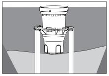
For concrete installation: Fill the hole around the fixture housing to 12" below the finished grade with clean fill dirt and tamp carefully to prevent settling of fixture. Pour concrete and finish as required flush with the top surface of the temporary cover.
