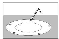
Remove faceplate using a 1/8" allen wrench. If 1. there is an optional accessory holder, carefully squeeze tabs on sides and gently pull from slots on OptiLock.
