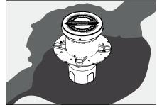
2. Place housing in hole. Align junction box in the path of the conduit trench.
