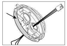
Wipe inside of housing where HydroLock plate will sit clean of debris before inserting patented HydroLock plate on to junction box. Align HydroLock plate with pins in housing and seat it firmly in place.
