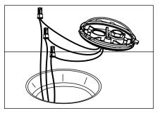
Make watertight connections using waterproof wire connectors (provided) to leads on the bottom of Patented HydroLock Barrier Plate Assembly. See wiring diagram.
