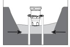
7. Per DIG-IT Guide, backfill the gap between the bottom of housing and bottom of hole with sand for drainage.
