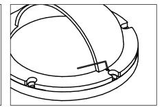
When set in final position, tighten two (2) #6-32 set screws using a 7/64" allen wrench. 5.
