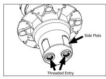
Connect branch conduit connectors (not included) to the junction box using either the threaded conduit entries on the bottom of the junction box or through holes drilled into the sides of the junction box.
