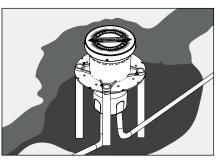
Pull primary branch circuit wiring into junction box.
