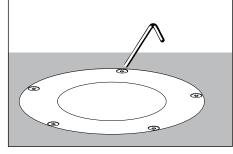
Install faceplate using a 1/8" allen wrench and hand-tighten the faceplate screws in a star 4. pattern to 30 in-lbs. min.
