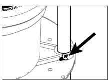
5. When housing is level, tighten screws on Stability Flange to secure housing to EMT. Remove excess EMT as needed.
