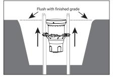
4. Raise housing on EMT so housing is flush with finished grade. Use a level to aid in housing installation.
