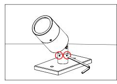
Use a 5/64" allen wrench to slightly loosen two (2) #8-32 stainless steel set screws on the stem for 360° aiming purpose.
