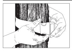
Remove canopy and/or fixture from MB2 housing. Use adjustable strap provided to attach MB2 housing to tree. Tighten by pulling on the adjustable strap until secure.
