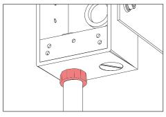
Run conduit (not included) to MB2 box location. MB2 box has four (4) 1/2" NPS tapped holes. Ensure unused tapped holes are plugged. Plugs are provided.
