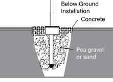
6. For below ground installation: Pour concrete to grade and flush with junction box.
