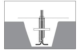
Pull low voltage wiring from remote transformer to power pipe. Allow for additional cable to make connections to fixture lead and future service. Place power pipe in hole.
