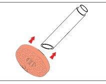
2. Slide stability flange onto power pipe. Use stability flange to aid in installation of power pipe.
