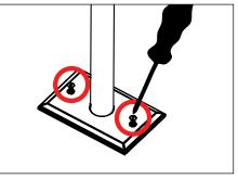
Attach box cover to junction box by tightening two (2) #6-32 stainless steel slotted screws to secure.
