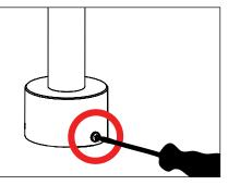
2. Place fixture on power pipe. Tighten three (3) #8-32 stainless steel round head phillips screws to secure to installed power pipe.
