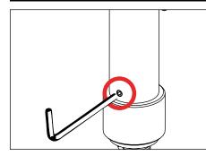
1. Use a 5/64" allen wrench to loosen #8-32 stainless steel set screw and remove cap.
