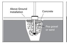
5. For above ground installation: Pour concrete below junction box.
