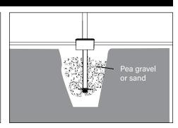
4. Back fill with pea gravel or sand prior to pour. Junction box can be installed above or below grade level.
