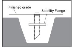
Excavate trench according to designed lighting plan. Dig hole a minimum of 24" deep and 10" wide to accommodate power pipe at desired fixture locations.
