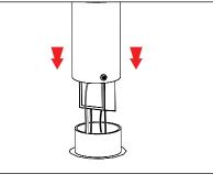
3. Place wires, connectors and transformer into transformer housing and attach to power pipe. Tighten three (3) #8-32 stainless steel round head phillips screws at transformer housing base to secure.
