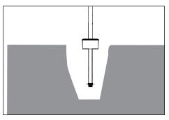
Excavate trench according to designed lighting plan. Dig hole a minimum of  $18^{\prime\prime}$  deep and  $10^{\prime\prime}$  wide 1. to accommodate anchor base at desired fixture locations.
