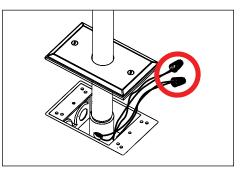
7. Make watertight connections from remote transformer to fixture leads using waterproof wire connectors. See wiring diagram.
