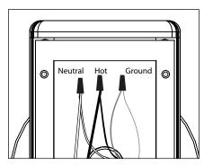
Use wire connectors (By Others) to connect transformer primary leads to branch circuit wires. Connect incoming ground to ground wire provided in UPM housing. See wiring diagram.
