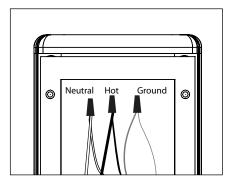
Use wire connectors (By Others) to connect 7. transformer primary leads to branch circuit wires. Connect incoming ground to ground wire provided in UPM housing. See wiring diagram.
