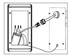
10. Connect transformer secondary leads to lamp 11. Make sure UPM body gasket is free of any dirt or leads using pre-wired factory connector.
