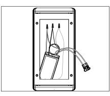
Remove the backing from adhesive tape on transformer, place in bottom of UPM housing void of any wiring and press firmly for five seconds to ensure good contact.
