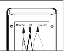
6. Use wire connectors (By Others) to connect transformer primary leads to branch circuit wires. Connect incoming ground to ground wire provided in UPM housing. See wiring diagram.
