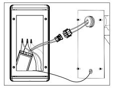
Connect transformer secondary leads to lamp 9 leads using pre-wired factory connector.
