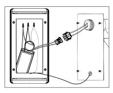
10. Connect transformer secondary leads to lamp leads using pre-wired factory connector.
