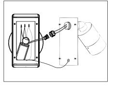
11. Connect transformer secondary leads to lamp leads using pre-wired factory connector.
