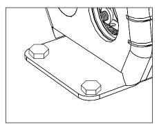
4. Attach the UPM housing at mounting brackets with ¼" fasteners (by others). Use suitable mounting hardware for surface.
