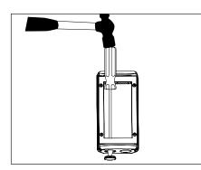
Remove Patented Knockout(s) as necessary from the inside of the UPM housing. Leave remaining unused knockouts in place to maintain seal.
