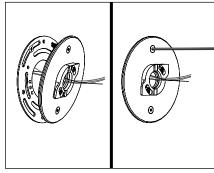
Feed branch circuit wiring through mounting plate with CamLock<sup>™</sup> assembly. Attach mounting plate with supplied (2) #10-24 stainless steel hex drive fasteners to universal ring using 1/8" allen wrench.
