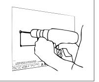
2. Drill holes into surface for  $\frac{1}{4}$ " fasteners (by others) on locations illustrated on template.
