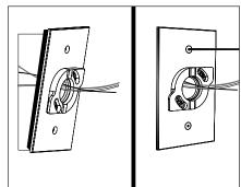
3. Feed branch circuit wiring through mounting plate with CamLock<sup>™</sup> assembly. Attach mounting plate with supplied (2) #6-32 stainless steel hex drive fasteners to recessed junction box using a 5/64" allen wrench.
