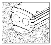
Anchor the UPM housing with mounting brackets provided using ¼" fasteners (By Others).
