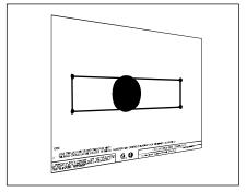
1. Place provided template in final mounting position according to designed lighting plan.
