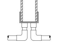
Connect conduit to the 1/2" conduit couplers attached to the bottom of the PowerPipe™. Place PowerPipe™ in hole.
