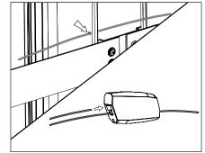
3. Optional Step on PM1 & PM2: Thread safety cable through hole on the back of the UPM housing. Feed safety cable through opposing ends of the connector. Pull on wires to assure the connection is secure. Leave enough slack in safety cable for tree growth. Adjustments can be made by pressing release spring with a pin or 3/64" allen tool.
