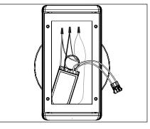
9. Remove the backing from adhesive tape on transformer, place in bottom of UPM housing void of any wiring and press firmly for five seconds to ensure good contact.
