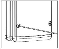
debris. Attach the faceplate by tightening the (4) #6-32 captive screws evenly to 6-9 in/lbs using a 5/64" allen wrench.
