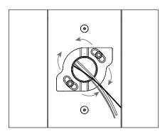
6. If UPM housing is not level, remove UPM housing; loosen but DO NOT REMOVE (2) #8-32 screws with 9/64" allen wrench on CamLock™ assembly. Adjust CamLock™ assembly up to 30° as needed to level. Tighten the screws and reattach UPM housing.
