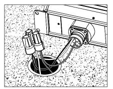
Use silicone filled wire nuts provided to connect branch circuit wiring to the anti-siphon (ASV<sup>m</sup>) wire pass-through located on the bottom of the UPM housing. See wiring diagram.
