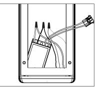
7. Remove the backing from adhesive tape on transformer, place in bottom of UPM body void of any wiring and press firmly for five seconds to ensure good contact.
