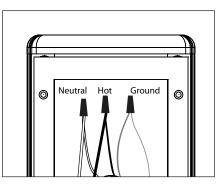
7. Use wire connectors (By Others) to connect transformer primary leads to branch circuit wires. Connect incoming ground to ground wire provided in UPM housing. See wiring diagram.
