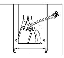
8. Remove the backing from adhesive tape on transformer, place in bottom of UPM housing void of any wiring and press firmly for five seconds to ensure good contact.
