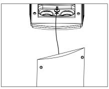
Attach tether wire under screw head at the base of the UPM housing and tighten. Slowly lower the faceplate until tether is taut.
