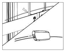
8. Optional Step on PM1 & PM2: Thread safety cable through hole on the back of the UPM housing. Feed safety cable through opposing ends of the connector. Pull on wires to assure the connection is secure. Leave enough slack in safety cable for tree growth. Adjustments can be made by pressing release spring with a pin or 3/64" allen tool.
