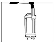
Remove Patented Knockout(s) as necessary from the inside of the UPM housing. Leave remaining unused knockouts in place to maintain seal.
