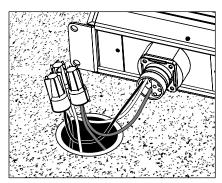
Use silicone filled wire nuts provided to connect branch circuit wiring to the anti-siphon (ASV™) wire pass-through located on the bottom of the UPM housing. See wiring diagram.
