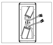
Remove the backing from adhesive tape on transformers, place in bottom of UPM body void of any wiring and press firmly for five seconds to ensure good contact.
