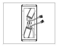
Remove the backing from adhesive tape on transformers, place in bottom of UPM housing void of any wiring and press firmly for five seconds to ensure good contact.
