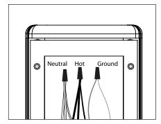
Use wire connectors (By Others) to connect both transformers primary leads to branch circuit wires. Connect incoming ground to ground wire provided in UPM housing. See wiring diagram.
