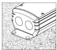
Anchor the UPM housing with mounting brackets provided using ¼" fasteners (By Others).
