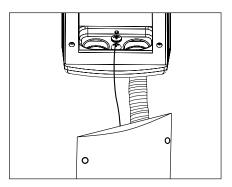
8. Attach tether wire under screw head at the base of the UPM housing and tighten. Slowly lower the faceplate until tether is taut.
