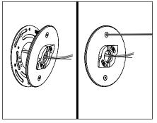
Feed branch circuit wiring through mounting plate with CamLock™ assembly. Attach mounting plate with supplied (2) #10-24 stainless steel hex drive fasteners to universal ring using 1/8" allen wrench.
