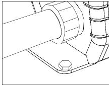
Connect 1/2" conduit connector through female threaded conduit entry
