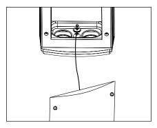
10. Attach tether wire under screw head at the base of the UPM housing. Slowly lower the faceplate
