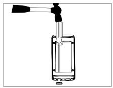
Remove Patented Knockout(s) as necessary from the inside of the UPM housing. Leave remaining unused knockouts in place to maintain seal.
