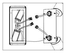
Connect transformers secondary leads to lamp leads using pre-wired factory connector.
