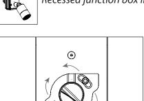
6. If UPM housing is not level, remove UPM housing; loosen but DO NOT REMOVE (2) #8-32 screws with 9/64" allen wrench on CamLock™ assembly. Adjust CamLock™ assembly up to 30° as needed to level. Tighten the screws and reattach UPM housing.
