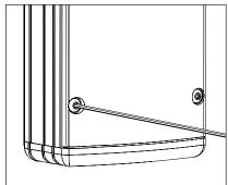
Make sure UPM body gasket is free of any dirt or debris. Attach the faceplate by tightening the (4) #6-32 captive screws evenly to 6-9 in/lbs using a 5/64" allen wrench.
