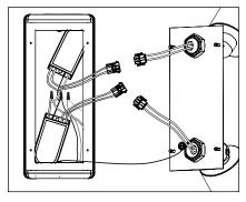
10. Connect transformers secondary leads to lamp 11. Make sure UPM body gasket is free of any dirt or leads using pre-wired factory connector.
