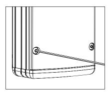
debris. Attach the faceplate by tightening the (4) #6-32 captive screws evenly to 6-9 in/lbs using a 5/64" allen wrench.
