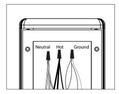
Use wire connectors (By Others) to connect branch circuit leads to lamp leads. Connect incoming ground and lamp ground to ground wire provided in UPM housing.
