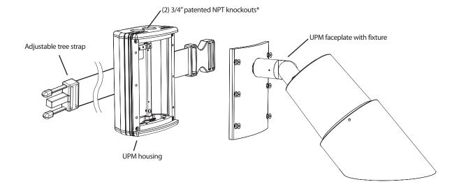
1. Remove Patented Knockout(s) as necessary from the inside of the UPM housing. Leave remaining unused knockouts in place to maintain seal.
