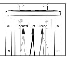
Use wire connectors (By Others) to connect branch circuit leads to lamp leads. Connect incoming ground and lamp ground to ground wire provided in UPM housing.
