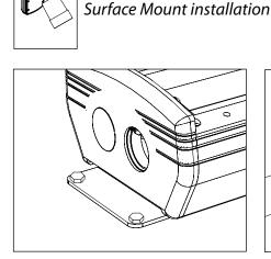
4. Attach the UPM housing at mounting brackets with 44'' fasteners (By Others). Use suitable mounting hardware for surface.
