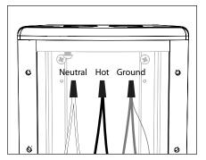
7. Use wire connectors (By Others) to connect branch circuit leads to lamp leads. Connect incoming ground and lamp ground to ground wire provided in UPM housing.
