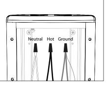
Use wire connectors (By Others) to connect branch circuit leads to lamp leads. Connect incoming ground and lamp ground to ground wire provided in UPM housing.
