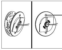
4. Feed branch circuit wiring through mounting plate with CamLock<sup>™</sup> assembly. Attach mounting plate with supplied (2) #10-24 stainless steel hex drive fasteners to universal mounting ring using 1/8" allen wrench.
