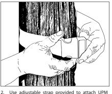
Use adjustable strap provided to attach UPM housing to tree. Tighten by pulling on the adjustable strap until secure. \* UPM is covered in whole or in part by US patent #6,940,012
