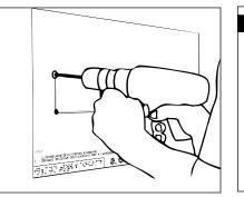
2. Drill holes into surface for ¼" fasteners (By Others) on locations illustrated on template.
