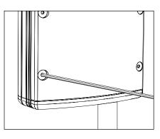
Make sure UPM housing gasket is free of any dirt or debris. Attach the faceplate by tightening the (6) #10-24 captive screws evenly to 30 in/lbs using a 1/8" allen wrench.
