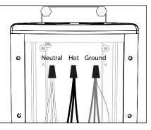
Use wire connectors (By Others) to connect branch circuit leads to lamp leads. Connect incoming ground and lamp grounds to ground wire provided in UPM housing.
