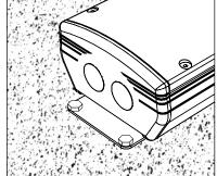
Anchor the UPM housing with mounting brackets provided using ¼" fasteners (By Others).
