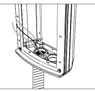
Pull branch circuit wiring necessary for installation (By Others.)
