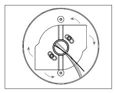
7. If UPM housing is not level, remove UPM housing; loosen but DO NOT REMOVE (2) #8-32 screws with 9/64" allen wrench on CamLock™ assembly. Adjust CamLock™ assembly up to 30° as needed to level. Tighten the screws and reattach UPM housing.
