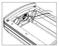
Pull branch circuit wiring necessary for installation (By Others.)
