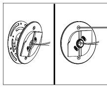
Feed branch circuit wiring through mounting plate with CamLock<sup>™</sup> assembly. Attach mounting plate with supplied (2) #10-24 stainless steel hex drive fasteners to universal mounting ring using 1/8" allen wrench.
