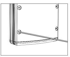
Make sure UPM housing gasket is free of any dirt or debris. Attach the faceplate by tightening the (6) #10-24 captive screws evenly to 30 in/lbs using a 1/8" allen wrench.
