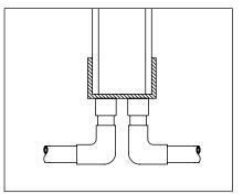
Connect conduit to the 1/2" conduit couplers attached to the bottom of the PowerPipe™. Place PowerPipe™ in hole.
