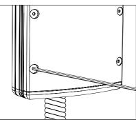
Make sure UPM housing gasket is free of any dirt or debris. Attach the faceplate by tightening the (6) #10-24 captive screws evenly to 30 in/lbs using a 1/8" allen wrench.
