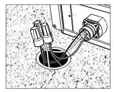
Use silicone filled wire nuts provided to connect branch circuit wiring to the anti-siphon (ASV<sup>m</sup>) wire pass-through located on the bottom of the UPM housing. See wiring diagram.
