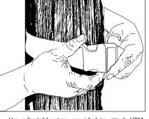
Use adjustable strap provided to attach UPM housing to tree. Tighten by pulling on the adjustable strap until secure.
