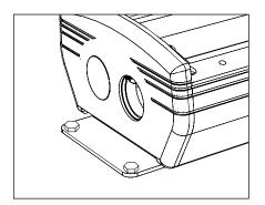
4. Attach the UPM housing at mounting brackets with  $\frac{1}{4}$ " fasteners (by others). Use suitable mounting hardware for surface.
