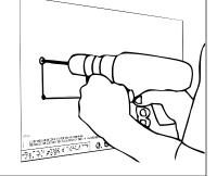
2. Drill holes into surface for  $^{1\!/}_{4''}$  fasteners (by others) on locations illustrated on template.
