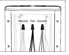
Use wire connectors (By Others) to connect branch circuit leads to lamp leads. Connect incoming ground and lamp grounds to ground wire provided in UPM housing.
