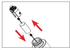
Pull the heat sink from the body to expose the LED board and Driver components. Utilize quick disconnects to change modular LED and driver components. Re-install the heat sink into body.
