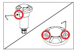
Replace faceplate assembly and tighten set screw. Re-Install fixture.
