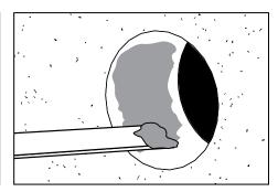
Use mixing stick to apply the epoxy to the interior of the 2-1/4" hole as shown.
