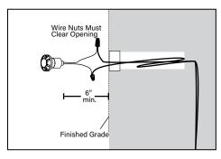
Pull low voltage wire through flush mount collar and make two low voltage connections using proper wire connectors (not included). Insert wires and fixture back into hole.
