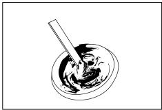
Drill 2-1/4" diameter hole, 3" deep minimum, for 2. Prepare epoxy according to instructions on packaging.
