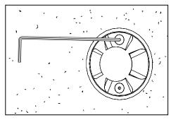
Mount faceplate to collar using two (2) #6-32 x 5/8" flat head cap screws (included) with a 5/64" allen wrench.
