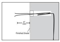
Supply low voltage wiring necessary for installation. Loop minimum of 6" of low voltage wire behind mounted collar to allow for fixture service.
