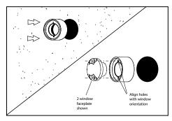
Fit flush mount collar into hole so it is flush with finished surface. Wipe off any excess adhesive.
