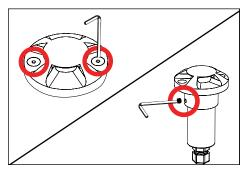
Loosen #8-32 set screw on faceplate assembly using a 5/64" allen wrench and remove. Loosen set screw on collar and remove.
