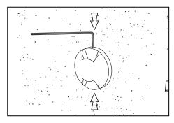
Loosen #8-32 set screws on the faceplate with a 5/64" allen wrench. Align window(s) to surface to be illuminated. Tighten set screws.
