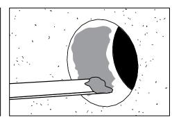
Use mixing stick to apply the epoxy to the interior of the 1-1/2" hole as shown.
