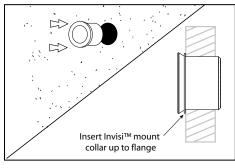
Fit Invisi™ mount collar into hole until flange comes in contact with building material. Wipe off any excess
