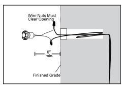
Pull low voltage wire through flush mount collar and make two low voltage connections using proper wire connectors (not included). Insert wires and fixture back into hole.
