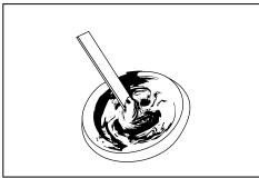
Drill 1-1/2" diameter hole, 3" deep minimum, for 2. Prepare epoxy according to instructions on packaging.
