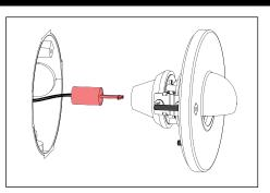
Disengage driver assembly by using quick disconnects. Replace driver assembly by using quick disconnects, then place driver back into junction box
