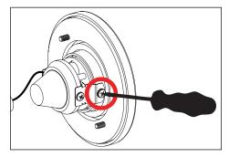
To aim adjustable bracket loosen the two (2) phillip screws attaching the adjustable bracket to the faceplate. Aim to desired position. Tighten two (2) phillip screws to lock in place when desired angle is set.
