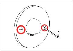
3. Mount faceplate using two (2) #10-24 screws with a 1/8" allen wrench. Tighten to compress gasket. Do not over tighten.
