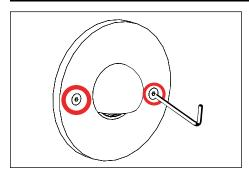
Use a 1/8" allen wrench to loosen #10-24 stainless 2. faceplate screws to remove faceplate.
