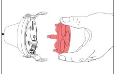
Space three fingers evenly around the optic and gently rock optic to remove. Insert new optic.
