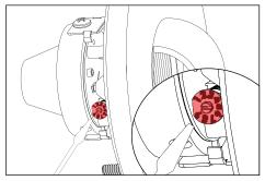
With flat head screw driver rotate dial to desired 3. Replace faceplate. lumen output.
