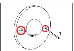
Mount faceplate using two (2) #10-24 screws with a 1/8" allen wrench. Tighten to compress gasket. Do not over tighten.
