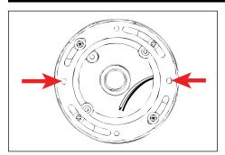
Remove #10-24 phillips screws from mounted back box. Install universal mounting ring (included with faceplate) using #10-24 screws onto back box. Align faceplate mounting holes to final mounting position.
