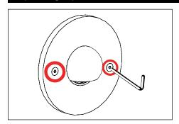
Remove faceplate by loosening #10-24 screws using a 1/8" allen wrench. Use phillips screwdriver to loosen heatsink from adjustable bracket.
