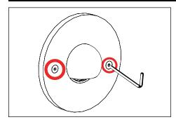
Use a 1/8" allen wrench to loosen #10-24 stainless faceplate screws to remove faceplate.
