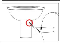
Use a 5/64" allen wrench to loosen #8-32 stainless set screw and remove cap.
