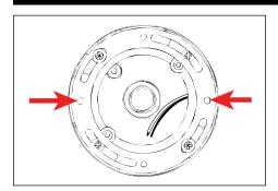
Install universal mounting ring (supplied with fixture) using #10-24 screws onto back box. Align fixture mounting holes to final mounting position. Universal mounting ring orientation determines fixture orientation.
