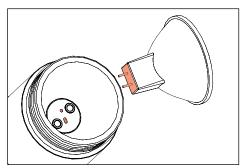
Firmly insert lamp pins into socket to make connection. Rocking motion maybe required.
