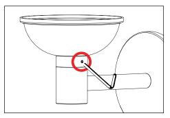
Use a 5/64" allen wrench on #8-32 stainless set screw to secure cap.
