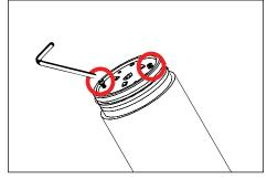
Use a 5/64" allen wrench to remove two (2) #2-56 socket head cap screws on LED board, grasp LED board and gently pull up to expose quick disconnect.
