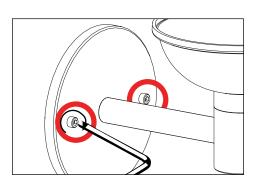
Using a 1/8" allen wrench mount fixture using two (2) #10-24 screws to installed back box.
