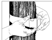
Use adjustable strap provided to attach UPM housing to tree. Tighten by pulling on the adjustable strap until secure.
