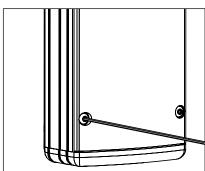
Make sure UPM body gasket is free of any dirt or debris. Attach the faceplate by tightening the (4) #6-32 captive screws evenly using a 5/64" Allen wrench.
