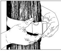
Use adjustable strap provided to attach UPM housing to tree. Tighten by pulling on the adjustable strap until secure.
