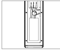
9. Remove the backing from adhesive tape on drivers, place in bottom of UPM housing void of any wiring and press firmly for five seconds to ensure good contact.
