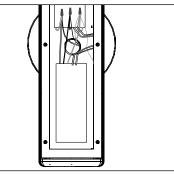
10. Remove the backing from adhesive tape on drivers, place in bottom of UPM housing void of any wiring and press firmly for five seconds to ensure good contact.
