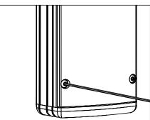
Make sure UPM body gasket is free of any dirt or debris. Attach the faceplate by tightening the (4) #6-32 captive screws evenly to 6-9 in-lbs using a 5/64" Allen wrench.
