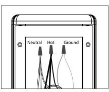
Use waterproof wire connectors (By Others) to connect both drivers primary leads to branch circuit wires. Connect incoming ground and drivers ground to ground wire provided in UPM housing. See wiring diagram.
