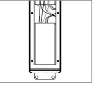
Remove the backing from adhesive tape on drivers, place in bottom of UPM housing void of any wiring and press firmly for five seconds to ensure good contact.
