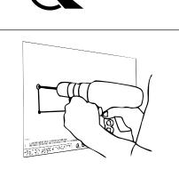
2. Drill holes into surface for ¼" fasteners (By Others) on locations required
