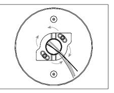
If UPM housing is not level, remove UPM housing; loosen but DO NOT REMOVE (2) #8-32 screws with 9/64" Allen wrench on CamLock<sup>™</sup> assembly. Adjust CamLock<sup>™</sup> assembly up to 30° as needed to level. Tighten the screws and reattach UPM housing.
