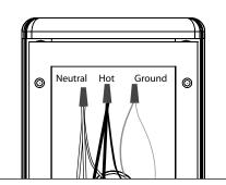
Use waterproof wire connectors (By Others) to connect both drivers primary leads to branch circuit wires. Connect incoming ground and drivers ground to ground wire provided in UPM housing. See wiring diagram.
