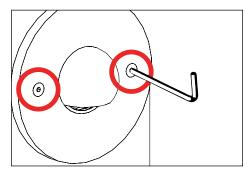
8. Use a 1/8" allen wrench to loosen #10-24 stainless faceplate screws to remove faceplate. for access to source
