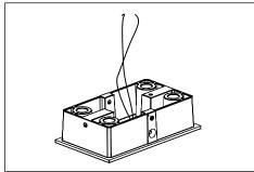
Pull low voltage wire or pull branch circuit wires necessary for installation through anchor base.
