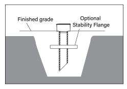
Excavate trench according to designed lighting plan. Dig hole a minimum of 18" deep and 10" wide to accommodate power pipe at desired fixture locations.
