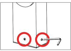
Place fixture on anchor base and tighten four (4) #10-32 stainless steel button head cap screws using a 1/8" allen wrench.
