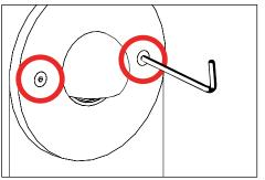
Use a 1/8" allen wrench to loosen #10-24 stainless faceplate screws to remove faceplate for access to
