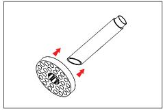
Slide optional stability flange onto power pipe. Use optional stability flange to aid in installation of power pipe.
