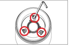
Use a .050" allen wrench to loosen three (3) set 3. screws holding optic holder and LED module.
