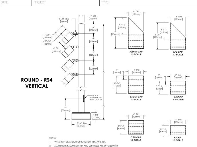
ALL HUME RS4 ALUMINUM 16ft AND 20ft POLES ARE OFFERED WITH A 100mph WINDSPEED RATING, WITH A 1.3 GUST FACTOR, UNDER 1994 AASHTO LTS-3; ALL OTHERS OFFERED WITH A 120mph RATING.
