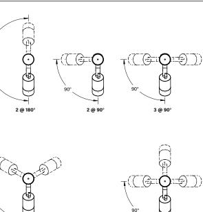
ALL HUME RS4 ALUMINUM 16ft AND 20ft POLES ARE OFFERED WITH A 100mph WINDSPEED RATING, WITH A 1.3 GUST FACTOR, UNDER 1994 AASHTO LTS-3; ALL OTHERS OFFERED WITH A 120mph RATING. 2.
